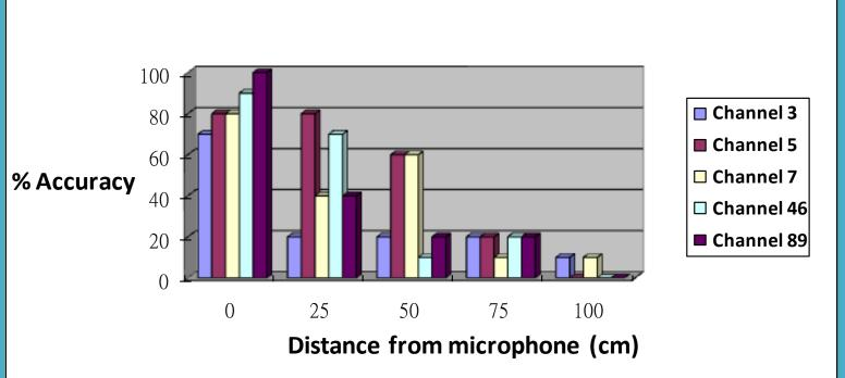
The graphs on the left show that our system yields very high accuracy when commands are given within a short distance from where the microphone is located. Testing was done with one male and one female voice sampled ten times per command, each.
